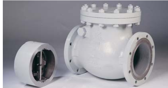
8" ANSI 150# Swing Check = 128kg 8" ANSI 150# Goodwin Wafer Check = 36kg
