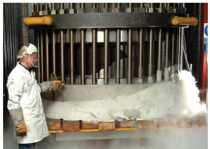
70" 150 lb valve cooling down for cryogenic test.
