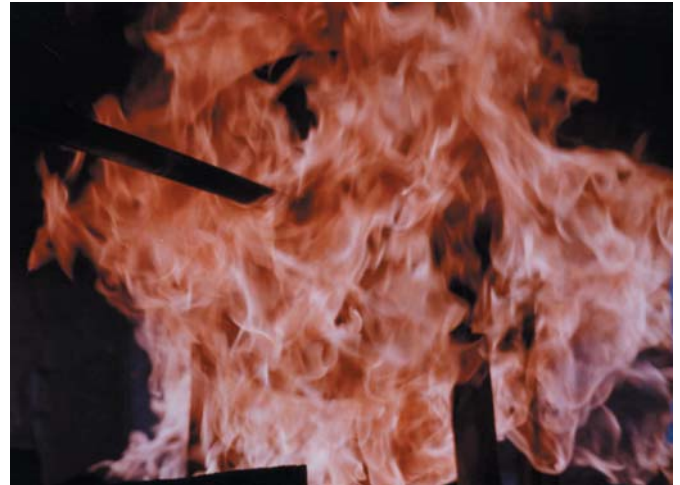
16" 600 lb BFR Flanged Check Valve undergoing firetest
