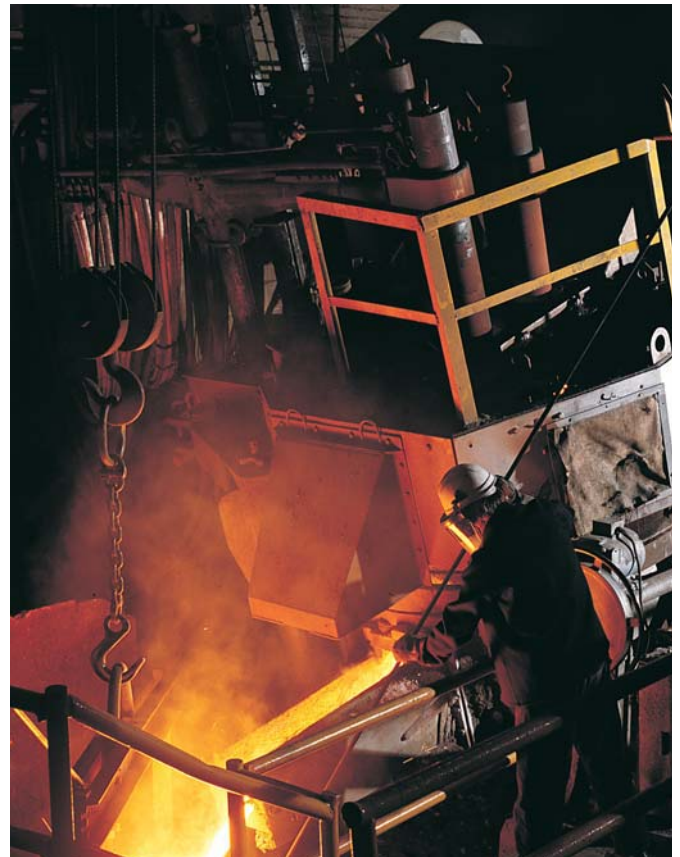
8 ton arc furnace at Goodwin Steel Castings
