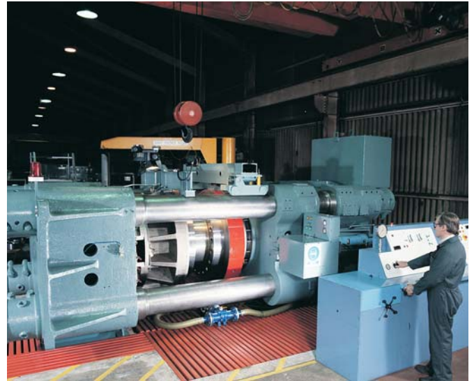
2500 tonne hydraulic test rig in Goodwin's Assembly bay
